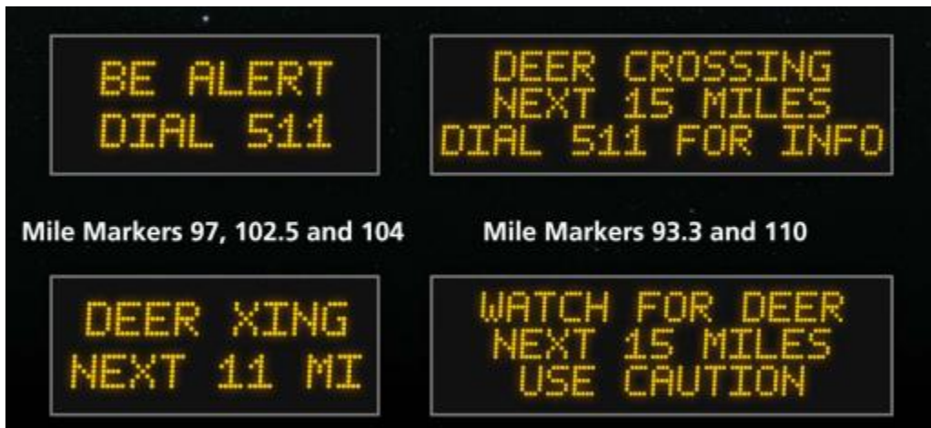
Figure 10. Example of a Changeable Message Sign with Deer Advisories To Alert And Educate Drivers which Have Been Found to Be Effective Deer-Vehicle Collision Reduction Tools. Example from a 2018 Virginia Transportation Research Council Report Titled “Effectiveness of Seasonal Deer Advisories on Changeable Message Signs as a Deer Crash Reduction Tool”
